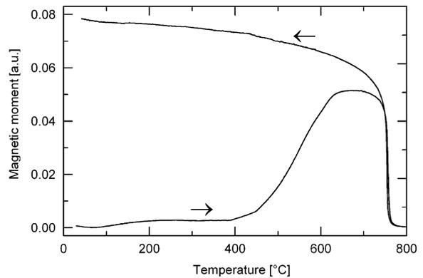
Fig. 2. Thermomagnetic curve of the as prepared  $\text{Fe}_{91.2}\text{W}_{8.8}$  amorphous powder measured at the field of  $3.98\text{ kA/m}$  with heating and cooling rate of  $4\text{ K/min}$  and  $30\text{ min}$  dwell time at  $800^\circ\text{C}$ .
