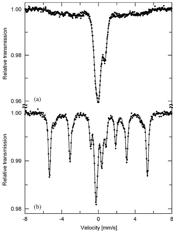
Fig. 1. Room temperature Mössbauer spectra of  $\text{Fe}_{91.2}\text{W}_{8.8}$  amorphous powder in the as prepared state (a) and after thermomagnetic curve measurement—as vacuum annealing  $800^\circ\text{C}/30\text{ min}$  (b).
