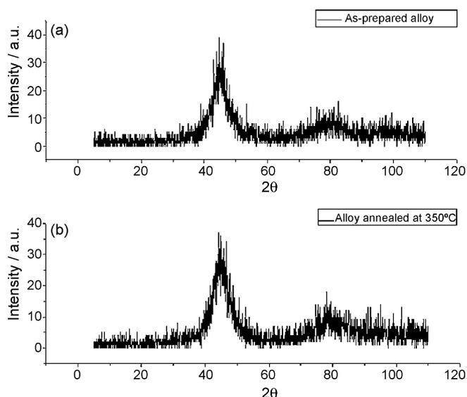
Fig. 2. XRD spectra of as-prepared alloy and sample of alloy annealed at  $350^\circ\text{C}$ .
