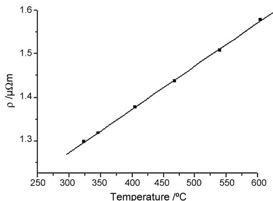
Fig. 6. Temperature dependence of the electric resistivity of the crystallized alloy.
