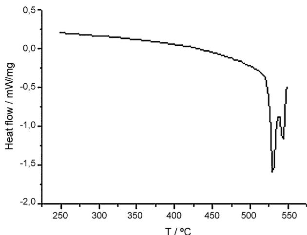
Fig. 1. DSC curve for  $\text{Fe}_{75}\text{Ni}_2\text{B}_{13}\text{Si}_8\text{C}_2$ ; heating rate  $5^\circ\text{C min}^{-1}$ .
