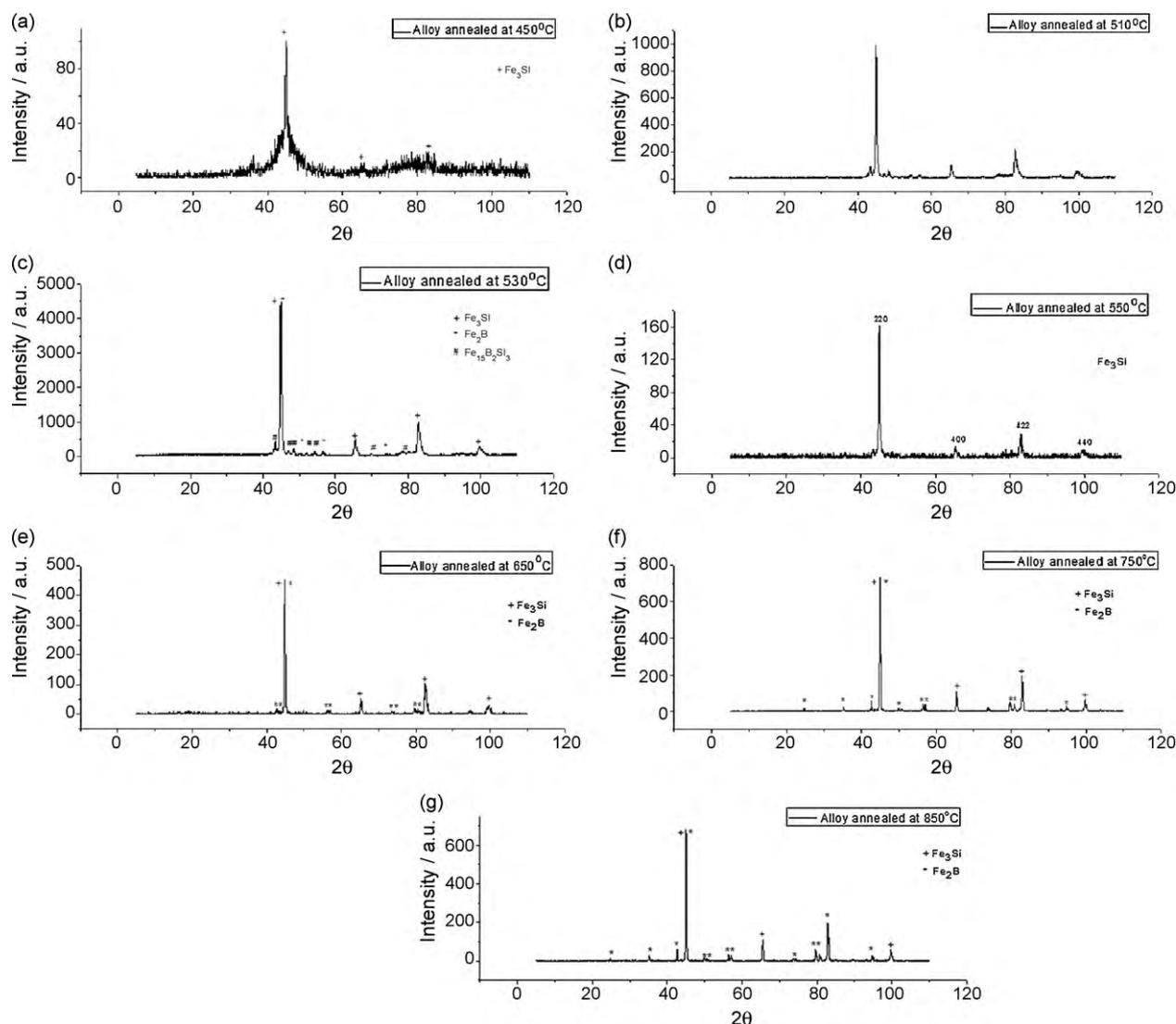
Fig. 3. XRD spectra of samples of alloy annealed at different temperatures.
