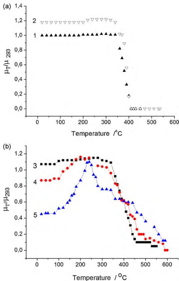
Fig. 4. (a) Temperature dependence of the relative magnetic susceptibility of alloy: first heating up to 450 °C and second heating up to 536 °C. (b) Temperature dependence of the relative magnetic susceptibility of alloy: third heating up to 550 °C; fourth heating up to 600 °C; and fifth heating up to 610 °C.
