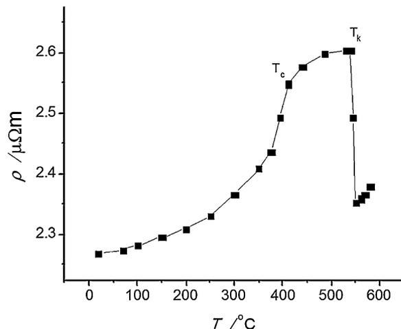
Fig. 5. Temperature dependence of the electrical resistivity of as-prepared alloy.
