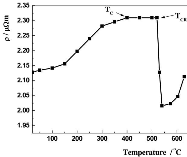
Fig. 7 Temperature dependence of the electrical resistivity of as-prepared alloy.
