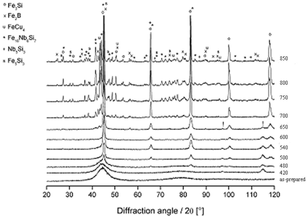
Figure 3 XRD patterns of  $\text{Fe}_{73.5}\text{Cu}_1\text{Nb}_3\text{Si}_{15.5}\text{B}_7$  as-prepared alloy and samples of alloy heated during 1 h at different temperatures as indicated in  $^{\circ}\text{C}$ .
