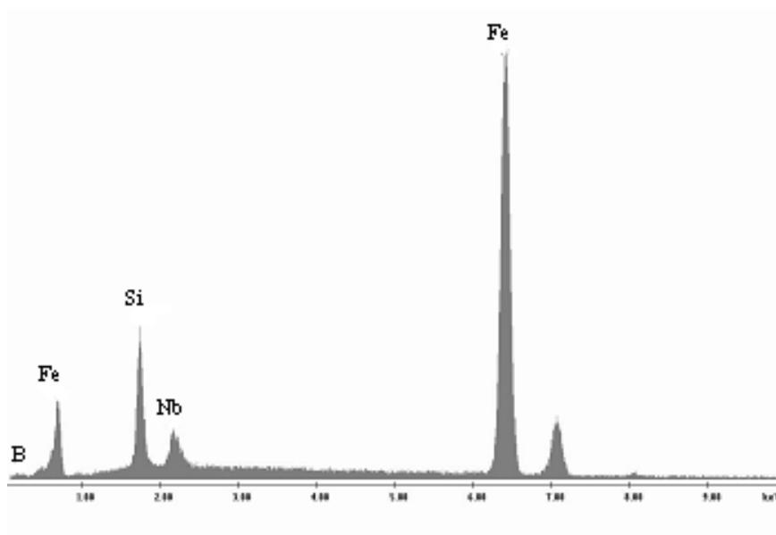
Fig. 1 EDAX spectrum of surface of as-prepared sample.
