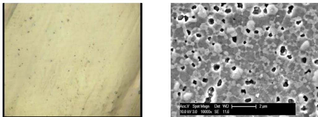
Figure 4 SEM micrograph (surface), as prepared alloy and sample of alloy annealed at 700 °C for 24 h.
