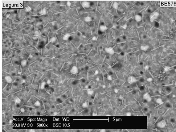
Figure 5. SEM micrograph (surface), sample after heat treatment at 850 °C for 24 h.
