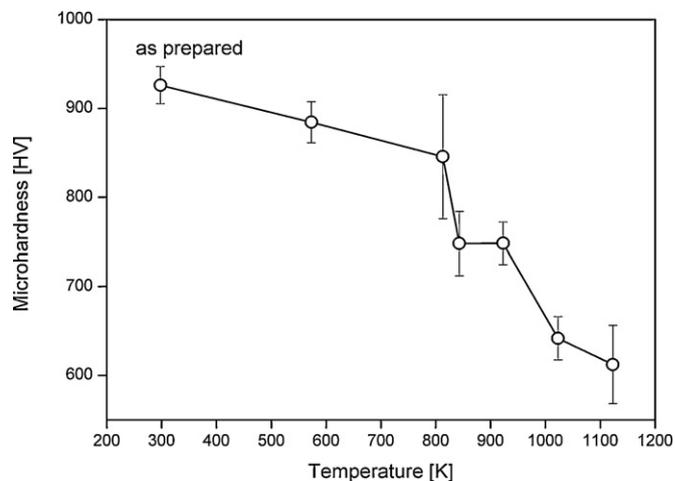
Fig. 10. Vickers microhardness (HV) mean values of the samples plotted as a function of the heating temperature together with the standard deviation error bars.
