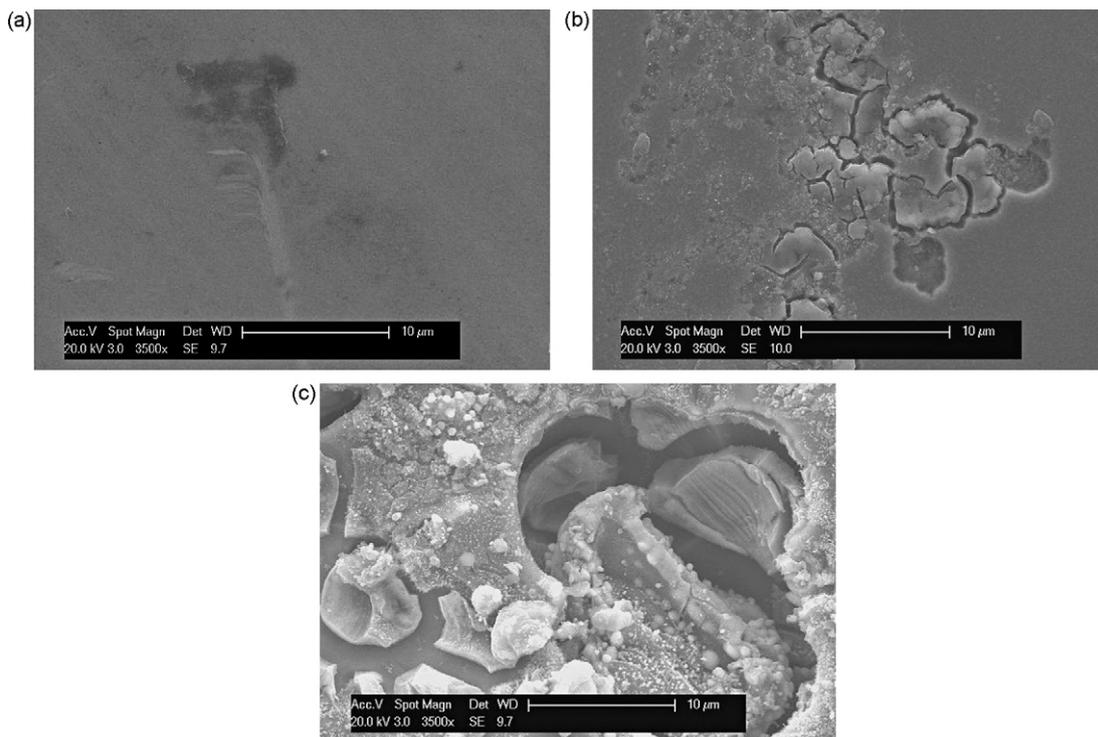
Fig. 7. (a) Scanning electron micrographs of the sample surfaces – as-prepared. (b) Scanning electron micrographs of the sample surfaces – after heat treatment at 753 K. (c) Scanning electron micrographs of the sample surfaces – after 923 K for 60 min.
