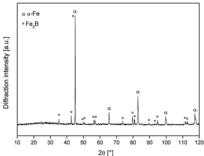
Fig. 3. XRD pattern of the sample heated at a temperature of 1123 K for 7 h.
