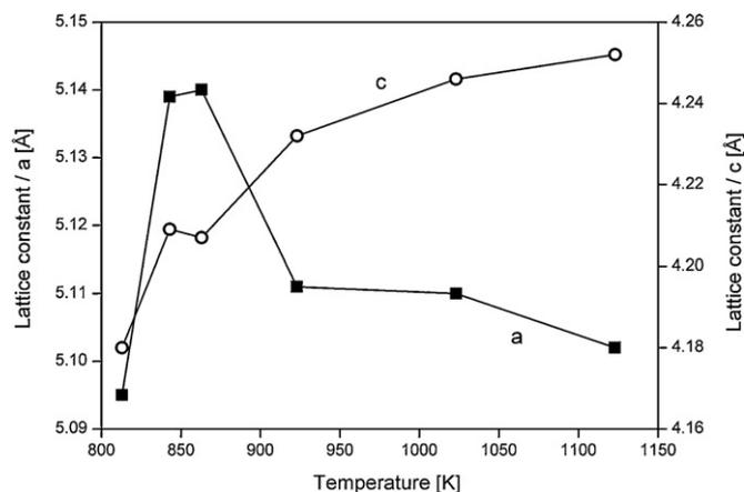
**Fig. 5.** Lattice constants *a* (indicated by squares) and *c* (indicated by circles) of the Fe<sub>2</sub>B phase as obtained by Rietveld refinement procedure plotted as a function of the heating temperature.
