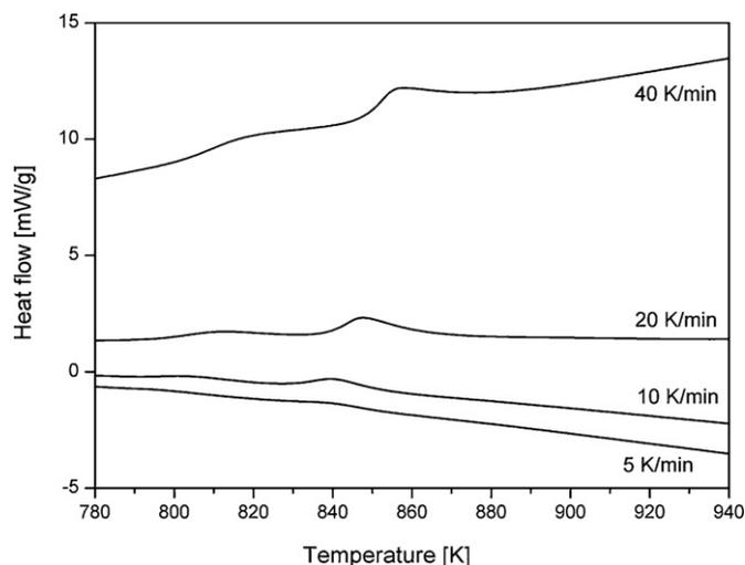
**Fig. 1.** DSC curves of the  $\text{Fe}_{89.8}\text{Ni}_{1.5}\text{Si}_{5.2}\text{B}_3\text{C}_{0.5}$  sample recorded at heating rates of 5, 10, 20, 40 K/min, respectively.
