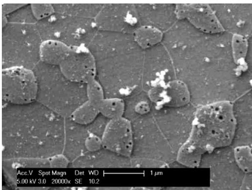
Fig. 8. Scanning electron micrograph of the polished surface of a  $\text{Fe}_{89.8}\text{Ni}_{1.5}\text{Si}_{5.2}\text{B}_3\text{C}_{0.5}$  sample heated at 1123 K for 7 h.
