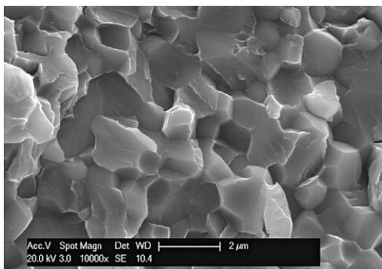
Fig. 9. Scanning electron micrograph of the cross-section (fracture surface) of a  $\text{Fe}_{89.8}\text{Ni}_{1.5}\text{Si}_{5.2}\text{B}_3\text{C}_{0.5}$  sample heated at 1123 K for 7 h.
