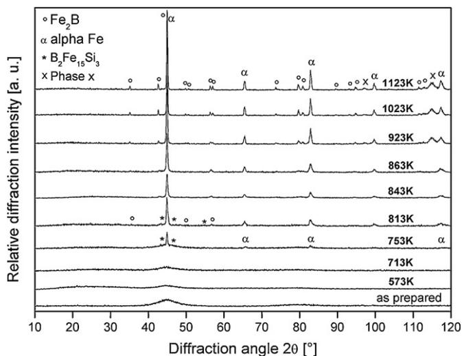
Fig. 2. XRD patterns of the as-prepared  $\text{Fe}_{89.8}\text{Ni}_{1.5}\text{Si}_{5.2}\text{B}_3\text{C}_{0.5}$  alloy as well as corresponding samples heated for 60 min at different temperatures at 573, 713, 753, 813, 843, 863, 923, 1023 and 1123 K.
