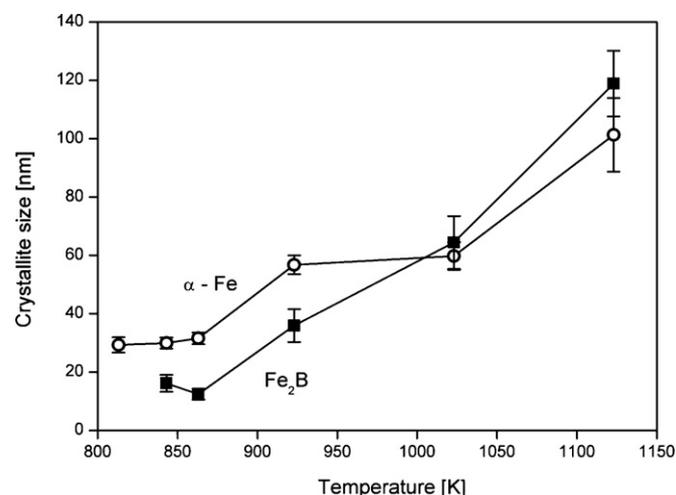
**Fig. 6.** Crystallite size as deduced from Rietveld refinement data for the α-Fe and Fe<sub>2</sub>B phases plotted as a function of the heating temperature.
