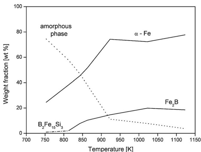
Fig. 4. Weight fractions of the observed crystalline phases as obtained by Rietveld refinement including the obtained amorphous weight content, plotted as a function of the heating temperature (1 h).
