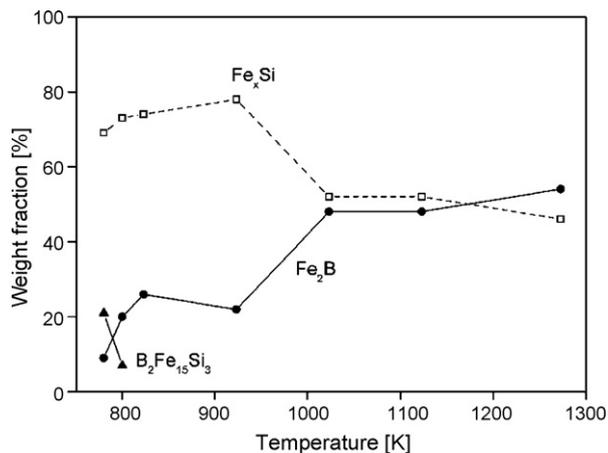
Fig. 5. Weight fraction as determined by Rietveld's refinement method.
