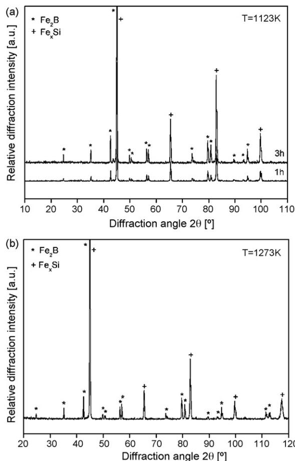
Fig. 3. X-ray diffraction patterns of  $\text{Fe}_{75}\text{Ni}_2\text{Si}_8\text{B}_{13}\text{C}_2$  alloy samples heated: (a) during 1 h and 3 h at 1123 K, and (b) during 3 h at 1273 K.
