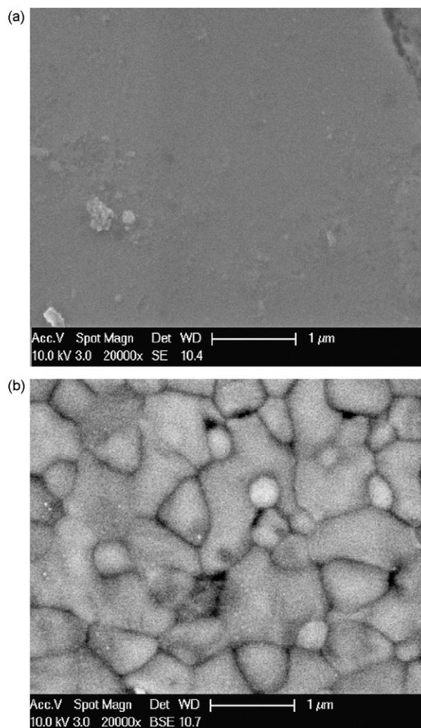
Fig. 7. Scanning electron micrograph images of the sample surface: (a) before heating and (b) after heat treatment at 1273 K during 1 h.
