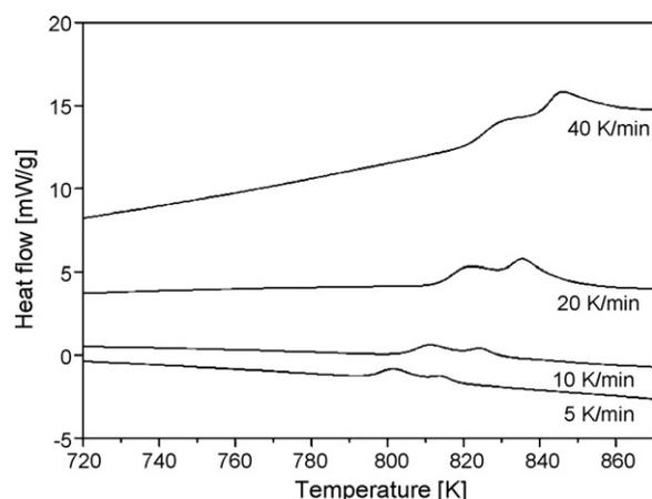
Fig. 1. Differential scanning calorimetry curves of alloy recorded at different heating rates.
