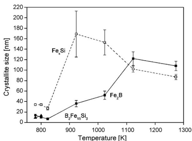
Fig. 6. Change of the crystallite size of phases formed during the isothermal heating of  $Fe_{75}Ni_2Si_8B_{13}C_2$  amorphous alloy.
