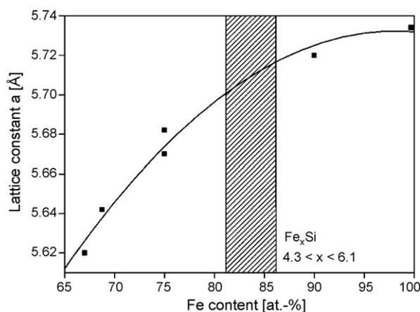
Fig. 4. Lattice constant for various  $\text{Fe}_x\text{Si}$  compounds as given in JCPDS database plotted as a function of the stoichiometric Fe content.
