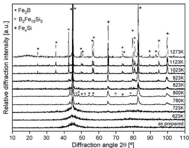
Fig. 2. X-ray diffraction patterns the as-prepared alloy and after thermal treatment at given temperatures.
