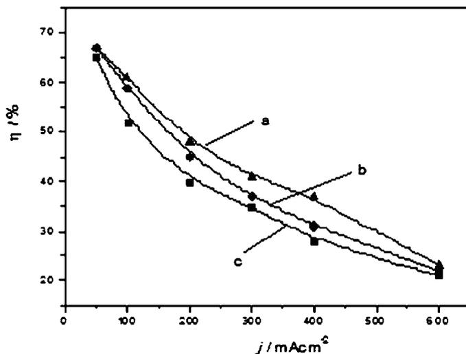
Figure 2. Current efficiency of the alloy deposition process at a Cu cathode vs. the current density for different composition of electrolyte: a)  $Ni^{2+}/Co^{2+} = 4$ ; b)  $Ni^{2+}/Co^{2+} = 1$  and c)  $Ni^{2+}/Co^{2+} = 0.25$ .
