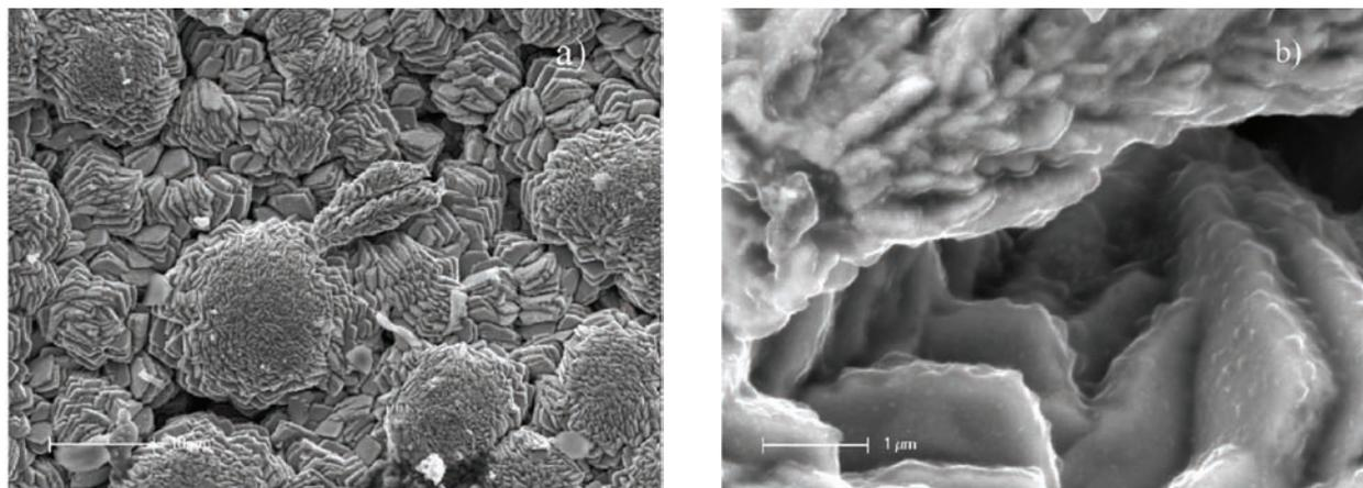
Figure 12. SEM micrographs of Ni-Co deposits on copper substrate prepared out of an electrolyte with concentration ratio  $Ni^{2+}/Co^{2+} = 0.25$ ,  $j = 65 mA cm^{-2}$  (alloy 2), upon annealing at 550 °C; a) magnification 2000 $\times$ , b) magnification 20000 $\times$  (SE, accelerating voltage 10 kV).
