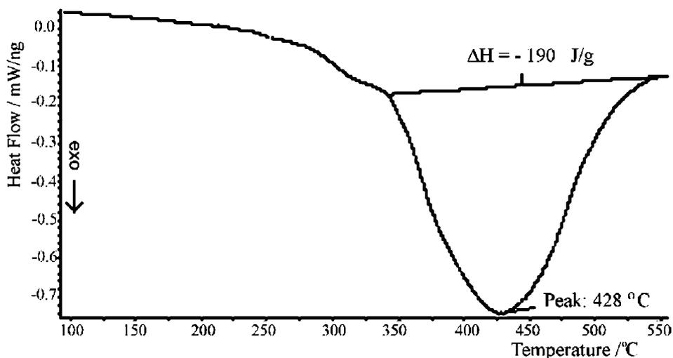
Figure 10. DSC of the alloy 2; heating rate:  $20 \text{ K min}^{-1}$ .
