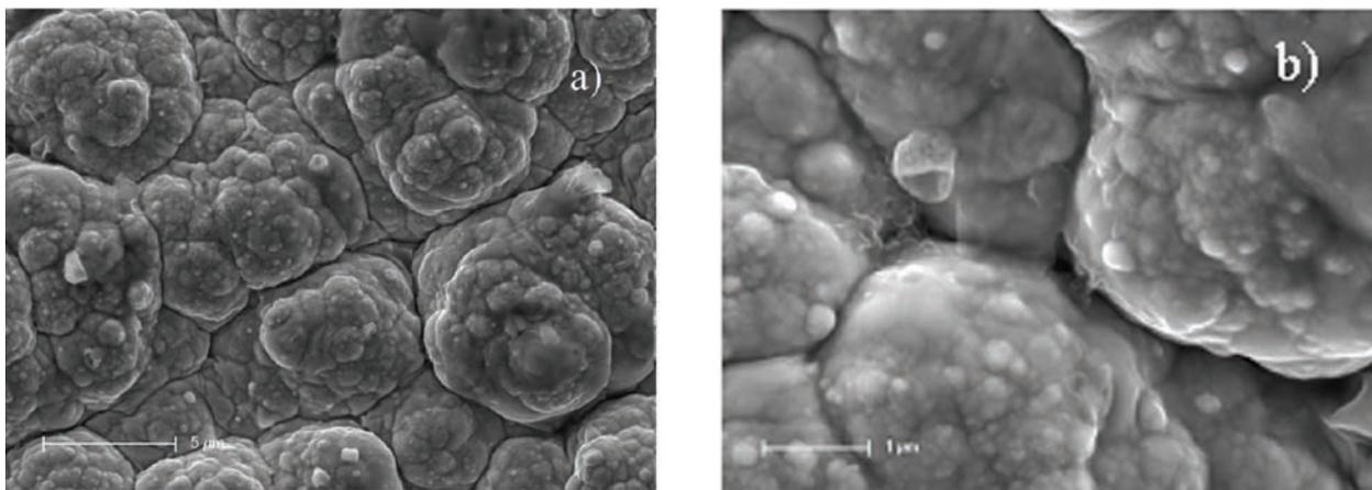
Figure 9. SEM micrographs of Ni–Co deposits on copper substrate prepared out of an electrolyte with concentration ratio  $Ni^{2+}/Co^{2+} = 4$ ,  $j = 65 \text{ mA cm}^{-2}$ , upon annealing at  $550 \text{ }^\circ\text{C}$ ; a) magnification  $5000\times$ ; b) magnification  $20000\times$  (SE, accelerating voltage:  $10 \text{ kV}$ ).
