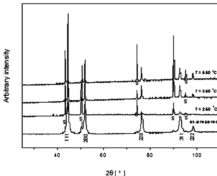
Figure 8. XRD patterns of alloy 1 as prepared and annealed at different temperatures.
