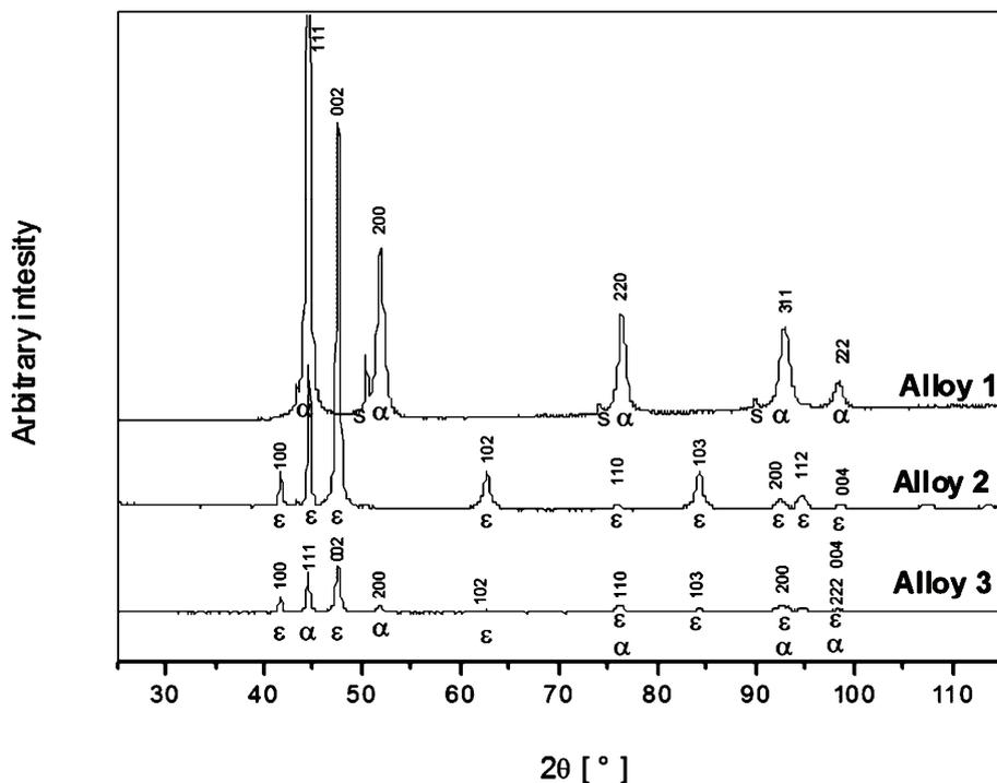
Figure 5. X-ray diffraction patterns of alloys 1, 2 and 3 ( $\alpha$  – reflections attributed to the  $\alpha$ -Ni;  $\epsilon$  – reflections attributed to the  $\epsilon$ -Co; S – reflection attributed to the Cu substrate).
