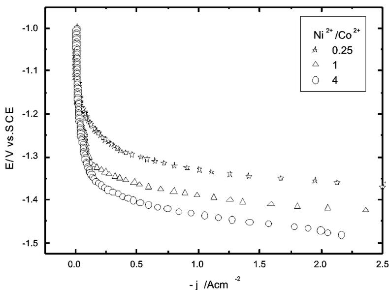
Figure 1. Polarization curves at the Cu cathode for the different compositions of the electrolyte: a)  $\text{Ni}^{2+}/\text{Co}^{2+} = 4$ ; b)  $\text{Ni}^{2+}/\text{Co}^{2+} = 1$  and c)  $\text{Ni}^{2+}/\text{Co}^{2+} = 0.25$ , sweep rate:  $1 \text{ mV s}^{-1}$ .
