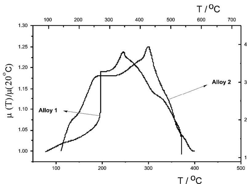
Figure 13. Temperature dependence of relative magnetic permeability of alloys.
