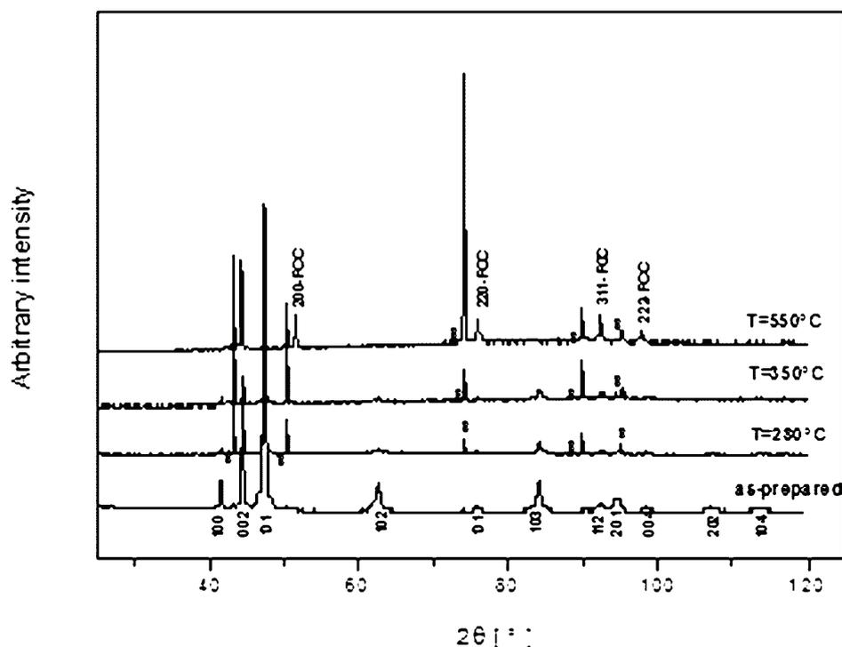
Figure 11. XRD patterns of alloy 2 as prepared as well as annealed at the different temperatures.
