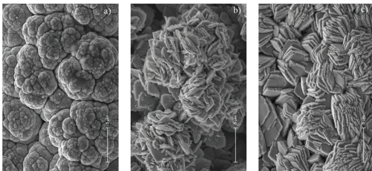
Figure 3. SEM micrographs of Ni–Co deposits obtained in the galvanostatic regime at a current density of  $65 \text{ mA cm}^{-2}$ . The concentration ratio  $Ni^{2+}/Co^{2+}$  in the electrolyte was: 4:1 (a), 1:1 (b) and 1:4 (c).
