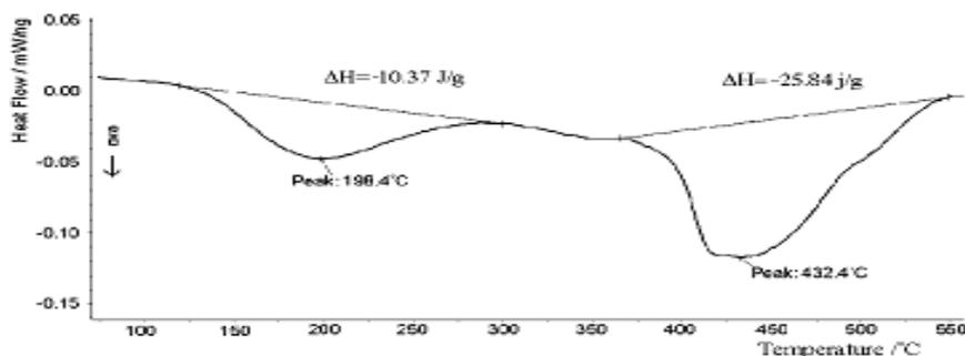
Figure 7. DSC of the alloy 1; heating rate 20 K min<sup>-1</sup>.
