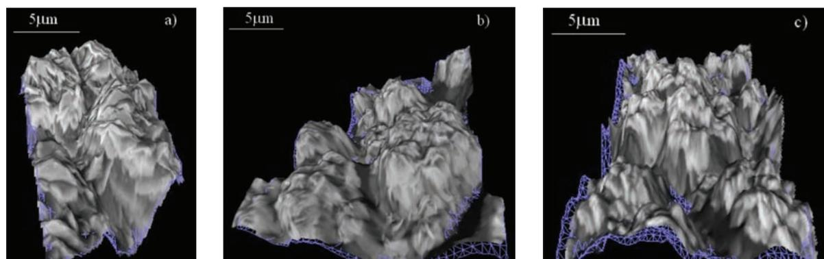
Figure 4. 3D SEM reconstructions of the surfaces of Ni–Co deposits from an electrolyte with concentration ratio  $Ni^{2+}:Co^{2+} = 1:1$  at different current densities: a) 65, b) 220 and c) 400  $mA\ cm^{-2}$ . (Figure 4a corresponds to Figure 3b).
