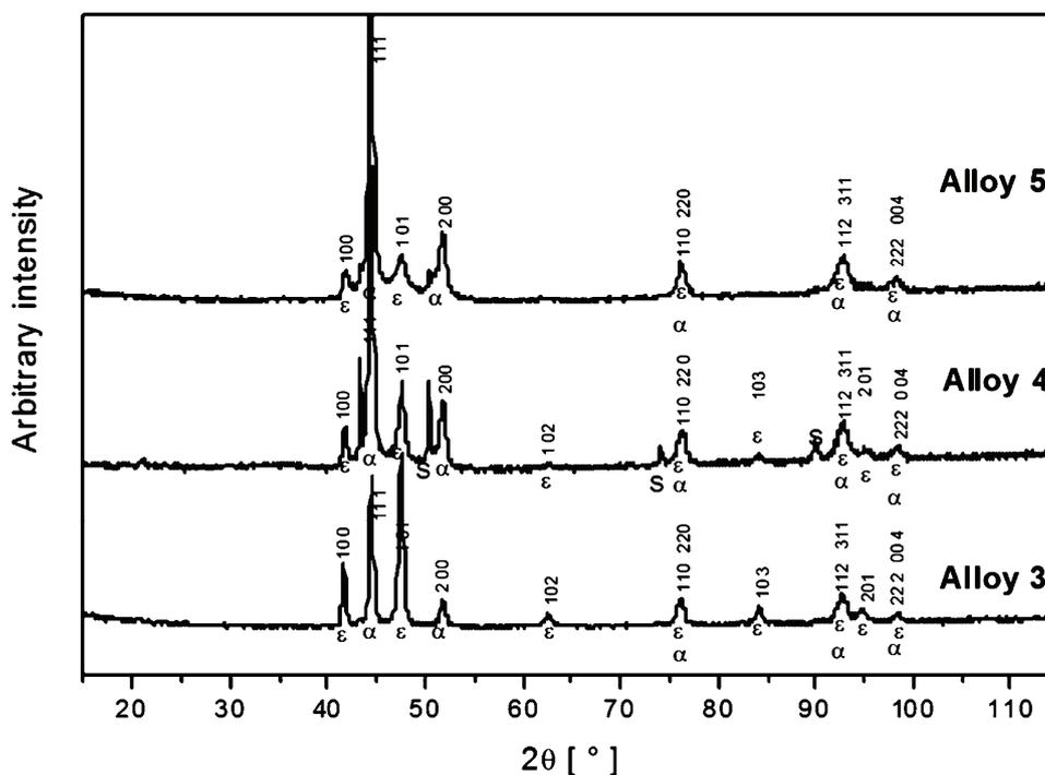
Figure 6. X-ray diffraction patterns of the alloys 3–5 ( $\alpha$  – reflections attributed to the  $\alpha$ -Ni;  $\epsilon$  – reflections attributed to the  $\epsilon$ -Co; S – reflection attributed to the Cu substrate).
